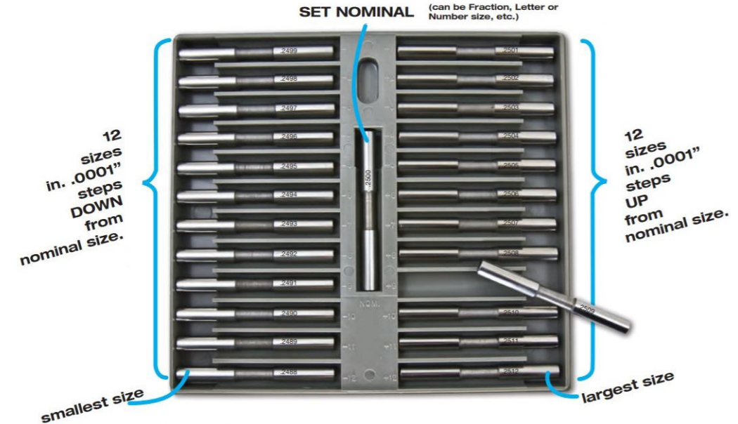
Illustrated: a TP25 Tenth set with a .2500" Nominal gage, center. 12 gages, left row, are in .0001" increments RANGING DOWNWARD from the Nominal size. Right row, 12 gages in .0001" increments RANGING UPWARD from the Nominal size
